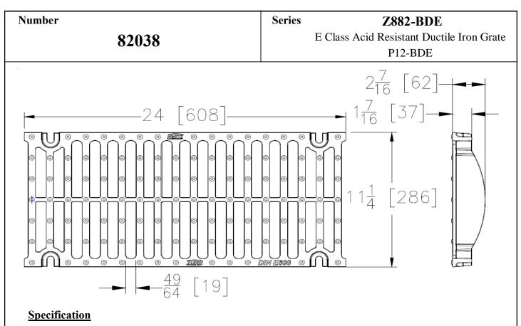
The Zurn P12-BDE Slotted Grate, Black Acid Resistant Epoxy Coated Ductile Iron Grate, is 11-1/4 inches wide by 24 inches long, weighing 19.8 lbs per linear foot. The grate has an open area of 60.3 square inches per linear foot, DIN Rating of E, ANSI Rating of Special-Duty, H-20 Load Rated and FAA Load Rated. Supplied by Trench Drain Supply.
